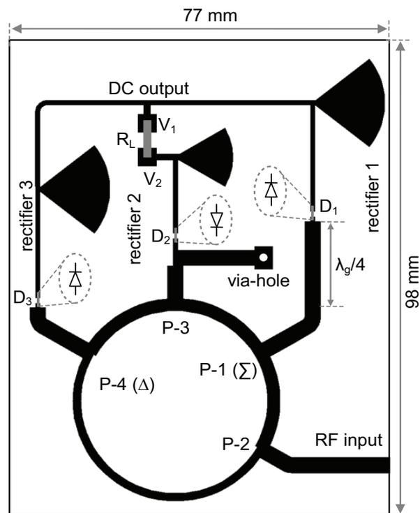
Figure 1. Layout of the dual-frequency microwave rectifier.
