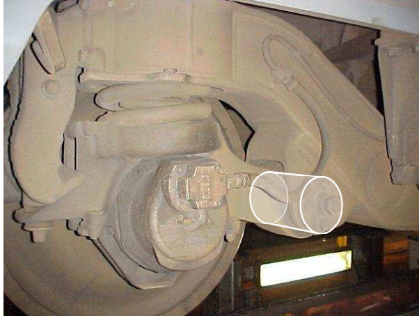
Figure 3. Picture of the train primary suspension. The location of the elastomeric stiffness is sketched as a white cylinder.
