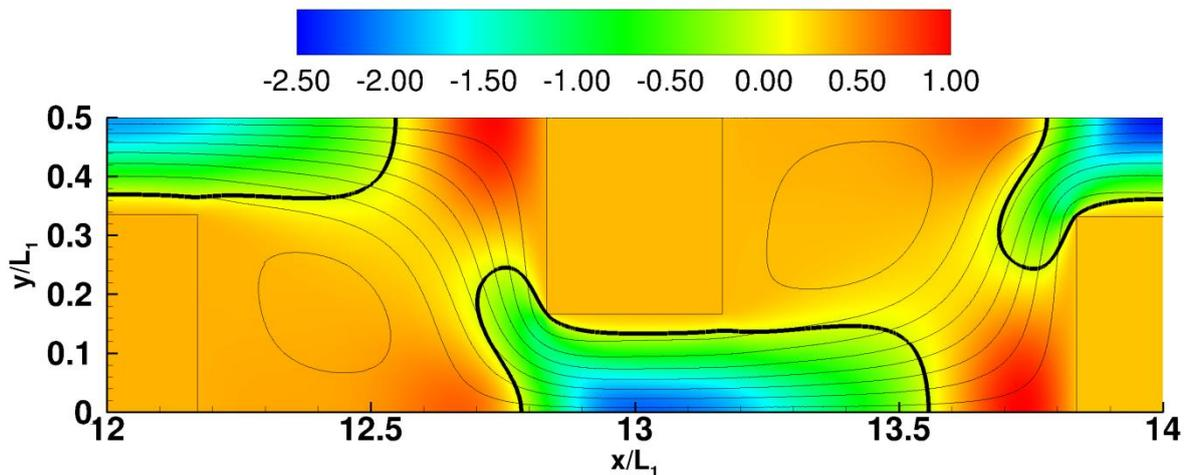
**Figure 4** : Difference between the local and mean fluid temperature, for the 7<sup>th</sup> REV. Stream lines are drawn with thin black lines. The thick lines indicate the places where the local temperature is equal to the average fluid temperature.
