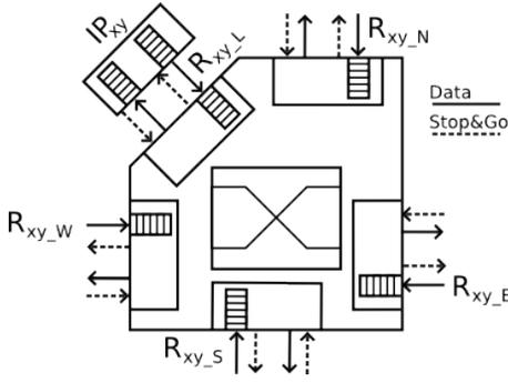
Fig. 1. Architecture of a NoC router  $R_{xy}$
