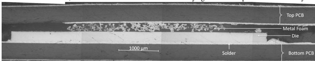
Fig. 2. Cross-sectional view of an embedded diode. The die is  $254\ \mu\text{m}$  thick.
