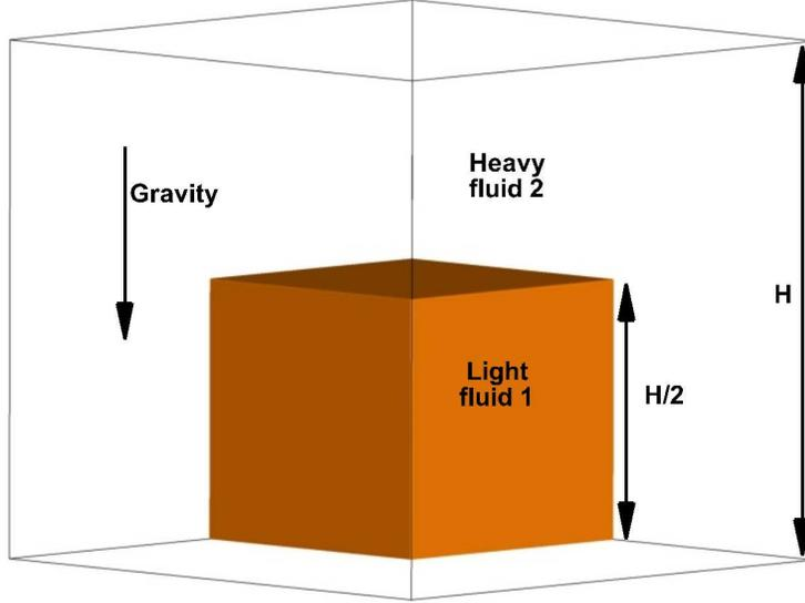
Figure 2: Definition sketch for the phase inversion benchmark in a closed box [2, 3, 15].
