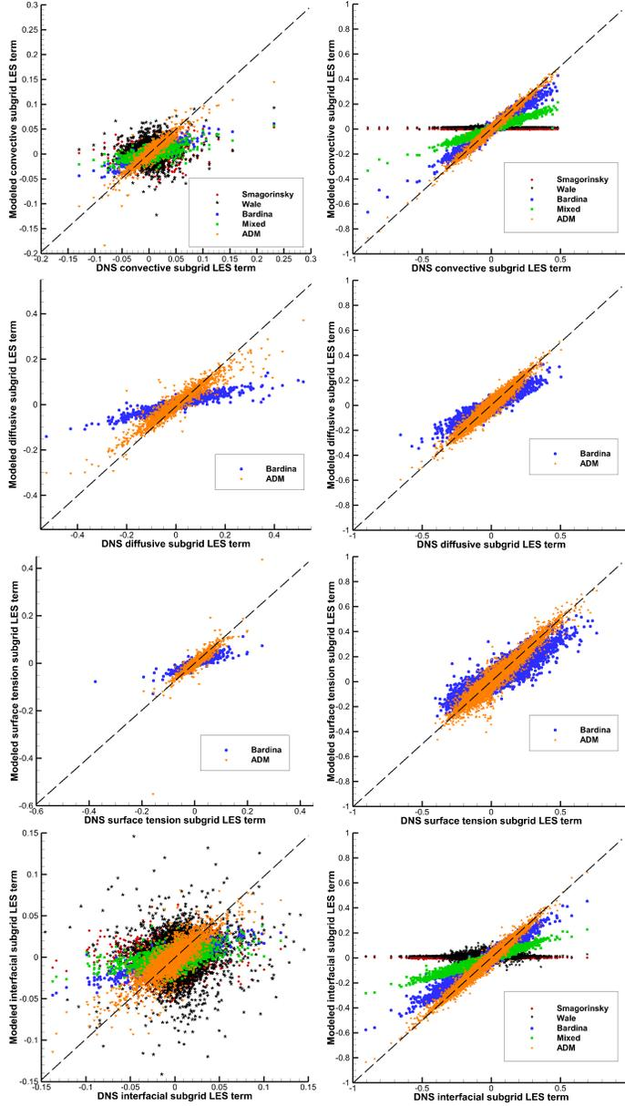
Figure 5: Spatial correlation of two-phase LES subgrid terms - The modeled terms are plotted according to the filtered DNS subgrid terms. A perfect modeling would be on the  $y=x$  line. Five LES models are considered: Smagorinsky [5], WALE [6], Bardina [7], Mixed model [8] and ADM [9]. Left column is for the one-fluid model whereas right column is for the multi-field approach.
