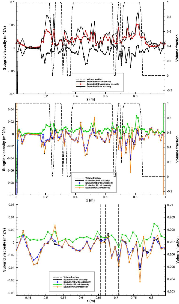
Figure 6: Comparison of equivalent turbulent viscosities obtained with DNS and LES OFM models, *i.e.* Smagorinsky [5], WALE [6], Bardina [7], Mixed model [8] and ADM [9]. The bottom line is a zoom on the middle plot. The results are plotted in a vertical line centered on  $[x = 0.6, y = 0.6]$ . The volume fraction is also plotted to locate interface position as  $C = 0.5$ .
