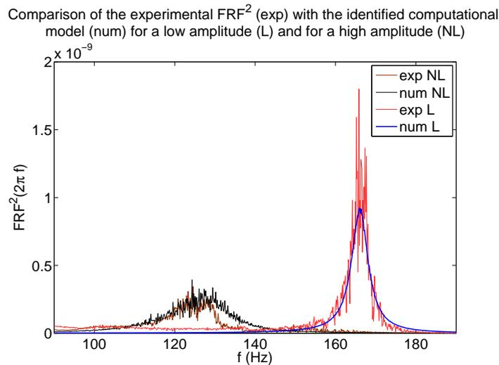
Figure 6: Comparison of the experimental FRF<sup>2</sup> (exp) with the identified computational model (num) for a low amplitude (L) and for a high amplitude (NL).
