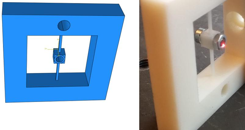
Figure 1: Design of the inclusion inserted in the frame (left figure) and its manufacturing with a 3D printing system (right figure).
