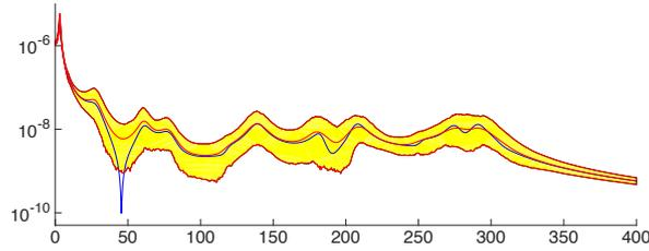
Figure 3: Graph of  $\nu \mapsto |\widehat{U}_1(2\pi\nu)|$  for the probabilistic model with causality in mean: 95% confidence region (yellow region) and mean value (red line). Graph of  $\nu \mapsto |\widehat{u}_1(2\pi\nu)|$  (blue line). Horizontal axis: frequency  $\nu$  in Hz.
