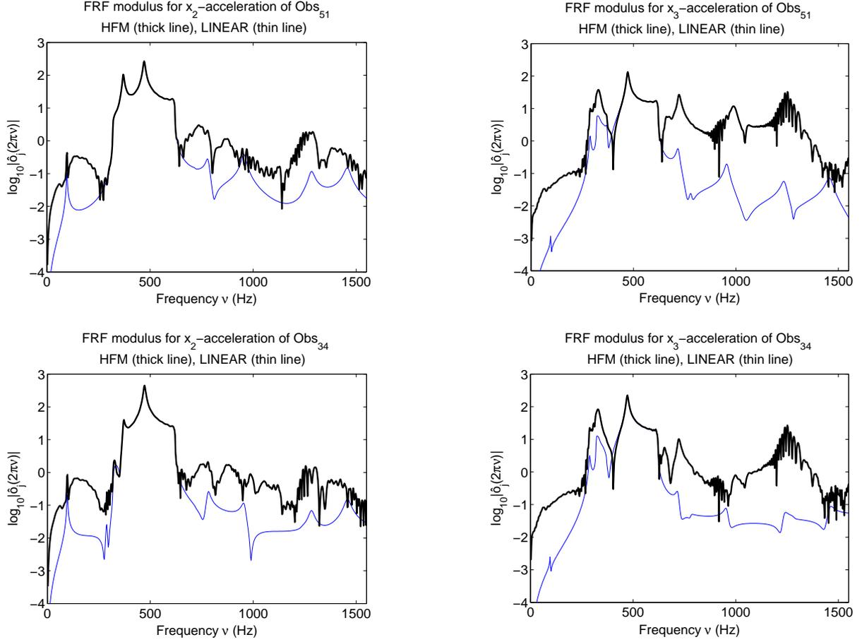
Figure 2: Graphs  $\nu \mapsto \log_{10}(|\hat{\delta}_j(2\pi\nu)|)$  computed with the HFM (thick lines) and with the LINEAR HFM (thin lines) for  $x_2$ - and  $x_3$ -accelerations of  $\text{Obs}_{51}$  (up left and up right figures), and for  $x_2$ - and  $x_3$ -accelerations of  $\text{Obs}_{34}$  (down left and down right figures).
