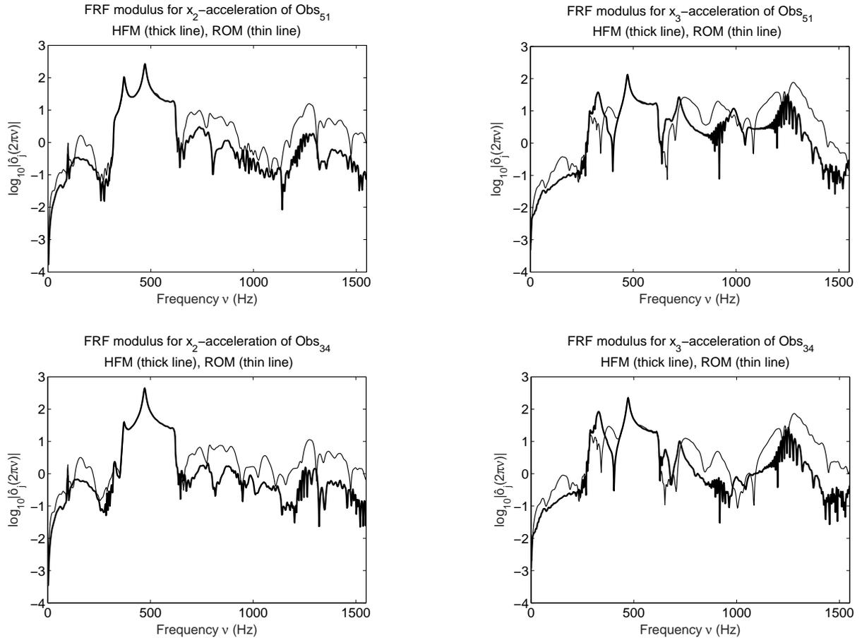
Figure 3: Graphs  $\nu \mapsto \log_{10}(|\hat{\delta}_j(2\pi\nu)|)$  computed with the HFM (thick lines) and graphs  $\nu \mapsto \log_{10}(|\hat{\delta}_j^{(n)}(2\pi\nu)|)$  computed with the ROM (thin lines) for  $x_2$ - and  $x_3$ -accelerations of Obs<sub>51</sub> (up left and up right figures), and for  $x_2$ - and  $x_3$ -accelerations of Obs<sub>34</sub> (down left and down right figures).
