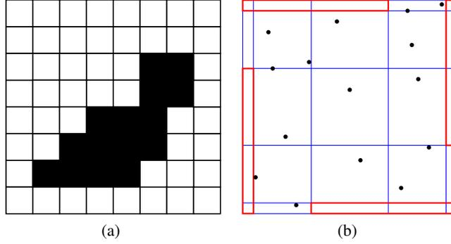
**Fig. 4.** (a) An initial finite set  $S \subset \mathbb{Z}^2$ , colored in black. (b) The remainder map image of  $S$ , i.e.  $\rho(\mathbf{p})$  for all  $\mathbf{p} \in S$ , under  $U$ — given by parameters  $(\arccos \frac{6}{37}, 0, \frac{2}{25})$ . Since no point  $\rho(\mathbf{p})$  lies within the non-injective zone  $\mathcal{F}$ , we have a *visual* proof that  $U$  restricted to  $S$  is injective.
