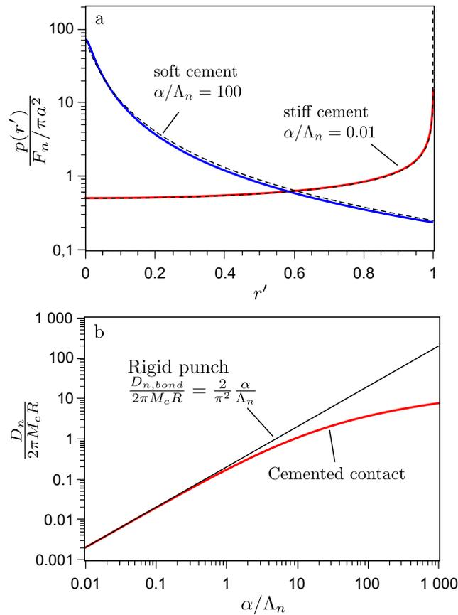
Figure 2. Contact-cement model predictions: (a) radial distribution of normal stresses in two cases: soft cement and stiff cement. The curves correspond to asymptotic solutions:  $1/2(1-r'^2)^{1/2}$  for stiff cement, and  $2/(r'+r'_c)^2$  for soft cement (b) Cemented contact stiffness as function of contact size  $\alpha$ .
