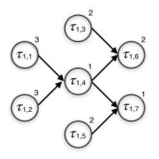
Figure 1: An example of a DAG task  $\tau_1$  which consists of 7 subtasks. The number on the upper right corner of each subtask represents its WCET and the arrows represent their precedence constraints.
