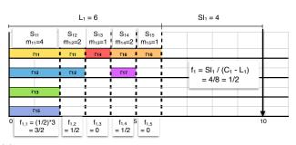
(a) The MTS representation of task  $\tau_1$  from Figure 1 showing the slack factors  $(f_i \& f_{i,j})$  derived using the stretching algorithm.
