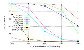
Figure 4: Comparison results of global EDF scheduling simulation between the DAG stretching algorithm and decomposition algorithm from [12]
