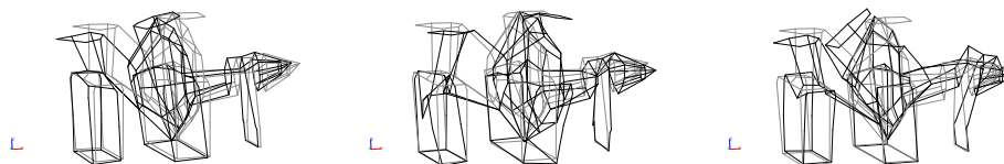
Figure 3: Pump 2: First three experimental mode shapes (Thick black line).
