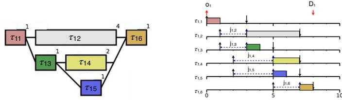
(a) A DAG task  $\tau_1$  consists of 6 subtasks with parameters:  $D_1 = 8$ ,  $C_1 = 10$ ,  $L_1 = 6$ .
