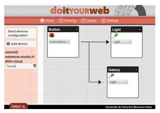
Fig. 13 The Design screen of  $BeC^3$  mashup tool, showing all devices. The behaviour chosen for each of them is indicated on the option list field. Publish-subscribe relations are shown with arrows. One node (TelosB) is available (on the left). Application is deployed with "Send devices configuration".
