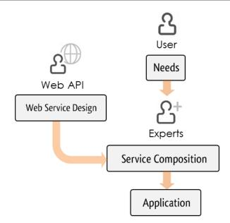
**Fig. 3** Usual SOC Design: A user expresses his needs to an Architect. The Architect builds the corresponding application using web-services offered by others programmers.
