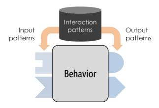
Fig. 5 A Behaviour in  $BeC^3$  is characterised by the way it interacts with others. Interaction Patterns describe typical interactions, and Behaviours inputs/output are restricted to Interaction Patterns.
