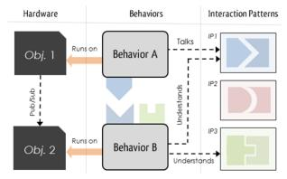
Fig. 9 Two Objects running  $BeC^3$  Behaviours. They interact because the two Behaviours correctly match the required Interaction Patterns. Object 2 runs a Behaviour that "understands" IP1 (needs it as an input), and optionally IP3. Object 1 runs a Behaviour that "talks" IP1. So publish/subscribe can be done.
