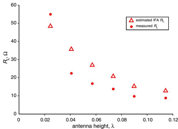
**Fig. 3** Estimation of IIFA loss resistance based on compensation theorem
