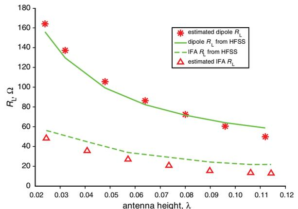
**Fig. 2** Loss resistance of half-wavelength dipole and IIFA
