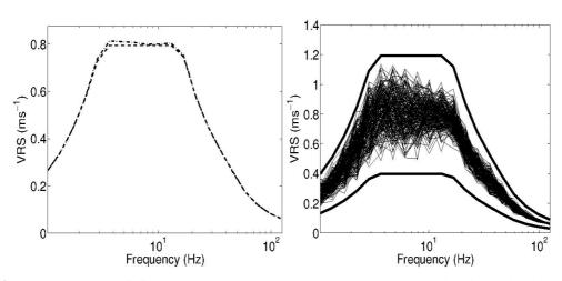
**Figure 2.** Random VRS. Left figure: mean value (the target) (dashed line) and estimation (mixed line). Right figure: 100 trajectories (thin lines), lower and upper envelops (thick lines).
