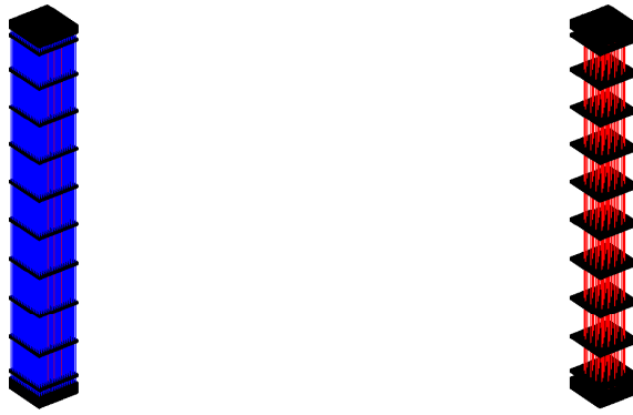
Figure 6 – Finite element mesh of a fuel assembly: Grids (black), fuel rods (blue) and guide tubes (red). Left figure: Complete fuel assembly. Right figure: Grids and guide tubes only.
