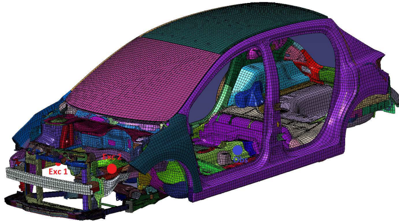
Figure 1 – The Finite Element model of an automotive vehicle
