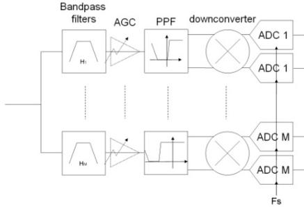
Figure 4. Subband splitting with analytic signals and downconversion
