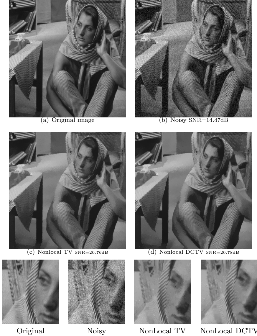
FIG. 3.3. Local and nonlocal denoising (Gaussian noise of variance \sigma^2 = 20 ). The nonlocal weights are computed using [13]. Regularization parameters used to obtain the best results: (e) \lambda = 0.048 (f) \lambda = 0.093 .
