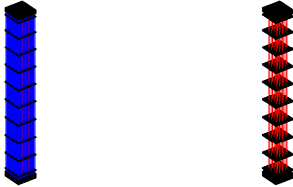
Figure 1: Finite element mesh of a fuel assembly: Grids (black), fuel rods (blue) and guide tubes (red). Left figure: Complete fuel assembly. Right figure: Grids and guide tubes only.
