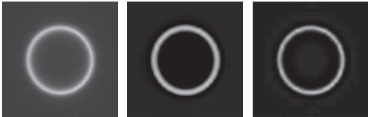
Figure 7. Restoration of the shell. Raw data (left), restored images using method 1 (center) and method 3 (right).
