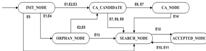
Fig. 3. The state-transition diagram of the clustering algorithm
