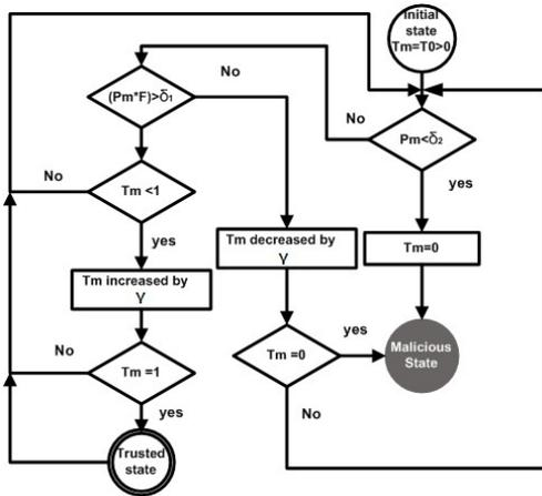
Fig. 2. The State-Transition Diagram of the Trust Model
