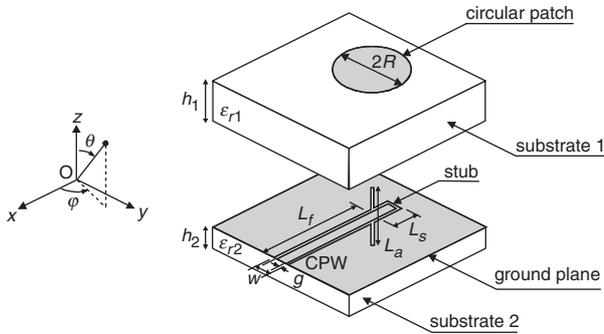
**Fig. 1** Geometry of circularly polarised microstrip antenna
