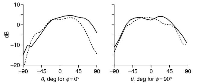
**Fig. 3** Measured radiation patterns at 5.99 GHz
