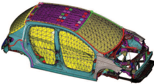
Figure 2: Finite element model of the vehicle structure and its internal acoustic cavity
