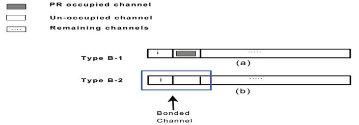
Fig. 3. Types of channels (Border Free Channel Case): (a) Type B-1, lower bandwidth category, and (b) Type B-2, higher bandwidth category.
