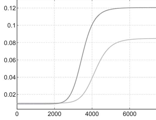
Figure 4: (Graph of function  $\nu \mapsto f(\nu, \mathbf{r}^{mod})$  (thick dark gray line) and  $\nu \mapsto f(\nu, \mathbf{r}^{pha})$  (thick light gray line) corresponding to the updated mean damping model. Horizontal axis is frequency  $\nu$  in Hz.
