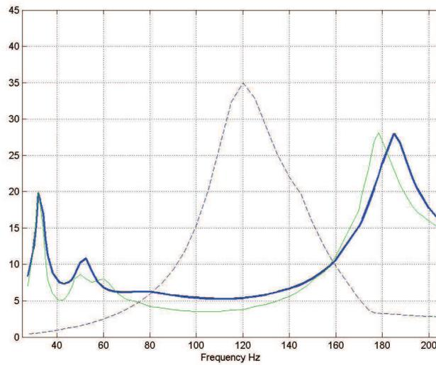
Figure 6: Graph of  $\omega \mapsto r(\omega)$  for the structure with trim: measurements (thin solid line) ; calculation (thick solid line) ; modal density  $\times 5.10^3$  (thin dashed line)
