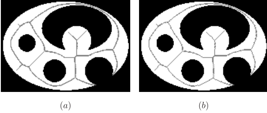
Fig. 11. A subset S of \mathbb{G}^2 (in white), (a) its \mathcal{K} -skeleton based on ends, (b) its \mathcal{K} -skeleton based on residues.
