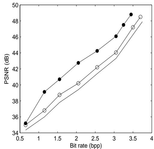
Figure 3: PSNR (in dB) versus the bit rate (bpp) after EZBC encoding for the SI pair "spot5-2": 5/3 for  $(I^{(l)}, I^{(e)})$  in solid line, 5/3 for  $(\tilde{I}, I^{(e)})$  in line with circle, VLS-II in dots.
