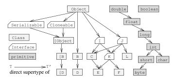
Fig. 1. Classes, interfaces, arrays and primitive types hierarchies
