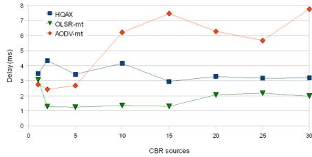
**Fig. 5.** Average Packet Delay / Number of CBR sources
