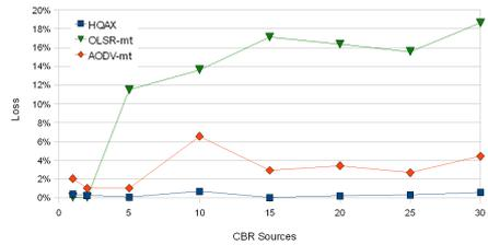
**Fig. 7.** Packet Loss / Number of CBR sources
