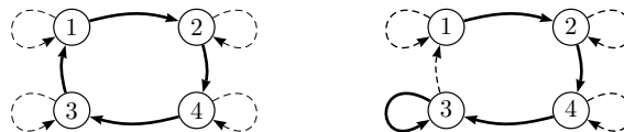
Fig. 1. Two complete deterministic automata labeled on A = \{a, b\} . A thick plain edge is an edge labeled by a while a thin dashed edge is an edge labeled by b . The automaton on the left is not synchronized. The one on the right is synchronized; for instance, the word aaa is a synchronizing word.
